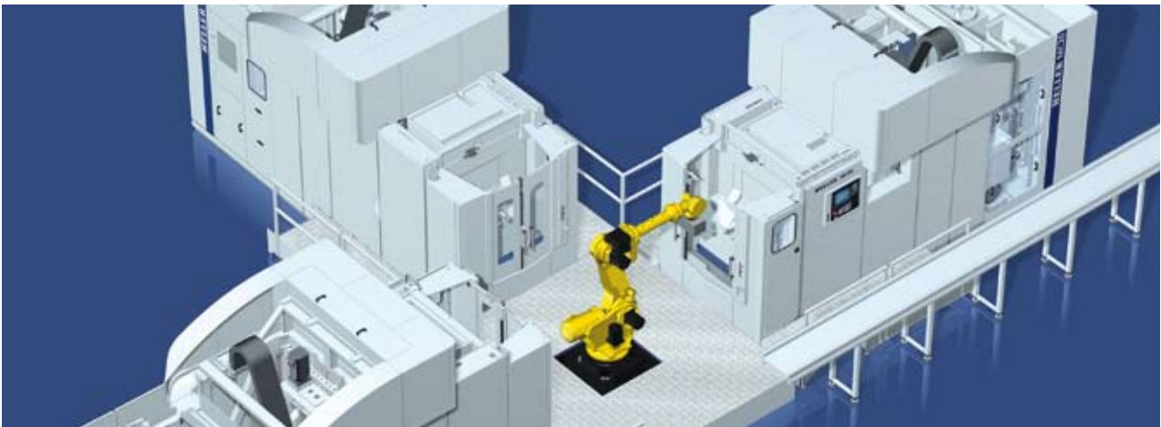
■ Stationary front loader: three machining modules linked via robot automation
