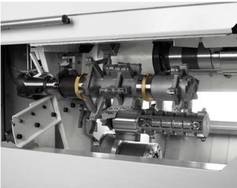
■ Disk-type magazine with oversize tools
