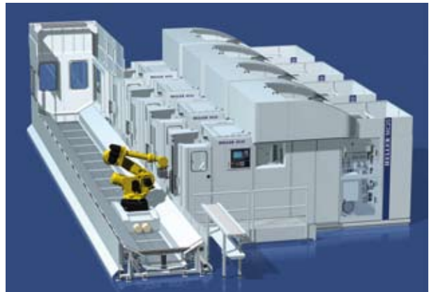
■ Mobile front loader: fully automatic loading via travelling robot
